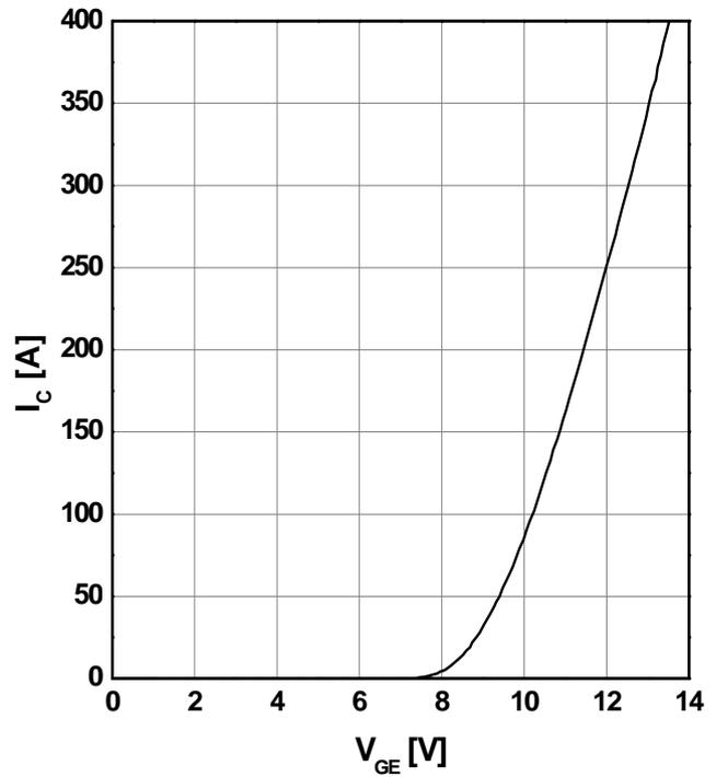
Fig2. Transfer Characteristics
