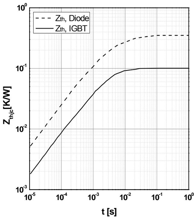
Fig7. Transient Thermal
