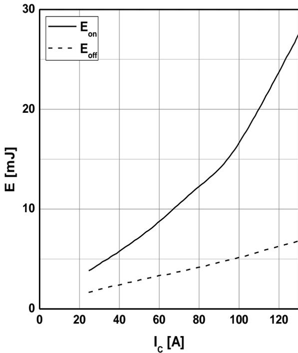
Fig3. Energy Loss vs. I<sub>c</sub>
