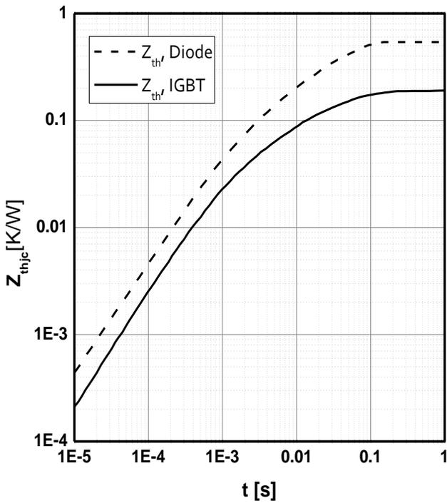
Fig7. Transient Thermal
