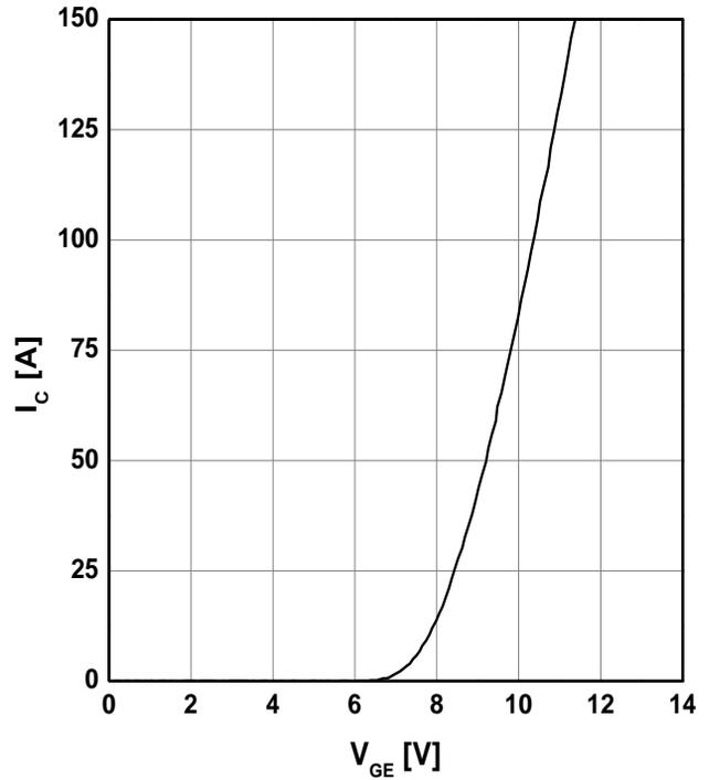
Fig2. Transfer Characteristics
