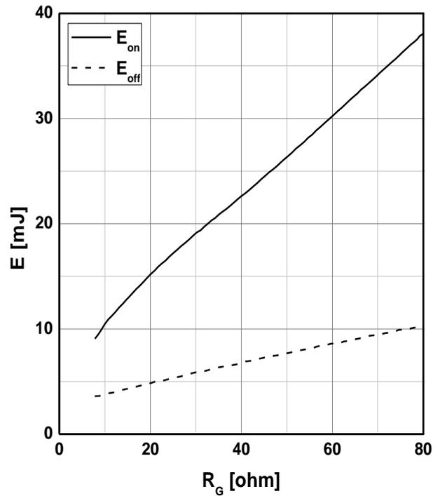
Fig4. Energy Loss vs. R<sub>G</sub>
